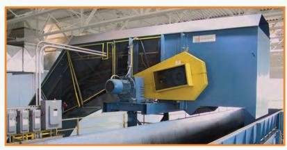
Discharge systems can range from simple discharge into a single container or trailer, to more complex systems featuring **two-position discharge chutes**, **rotary chutes** and **shuttle conveyor systems**.
