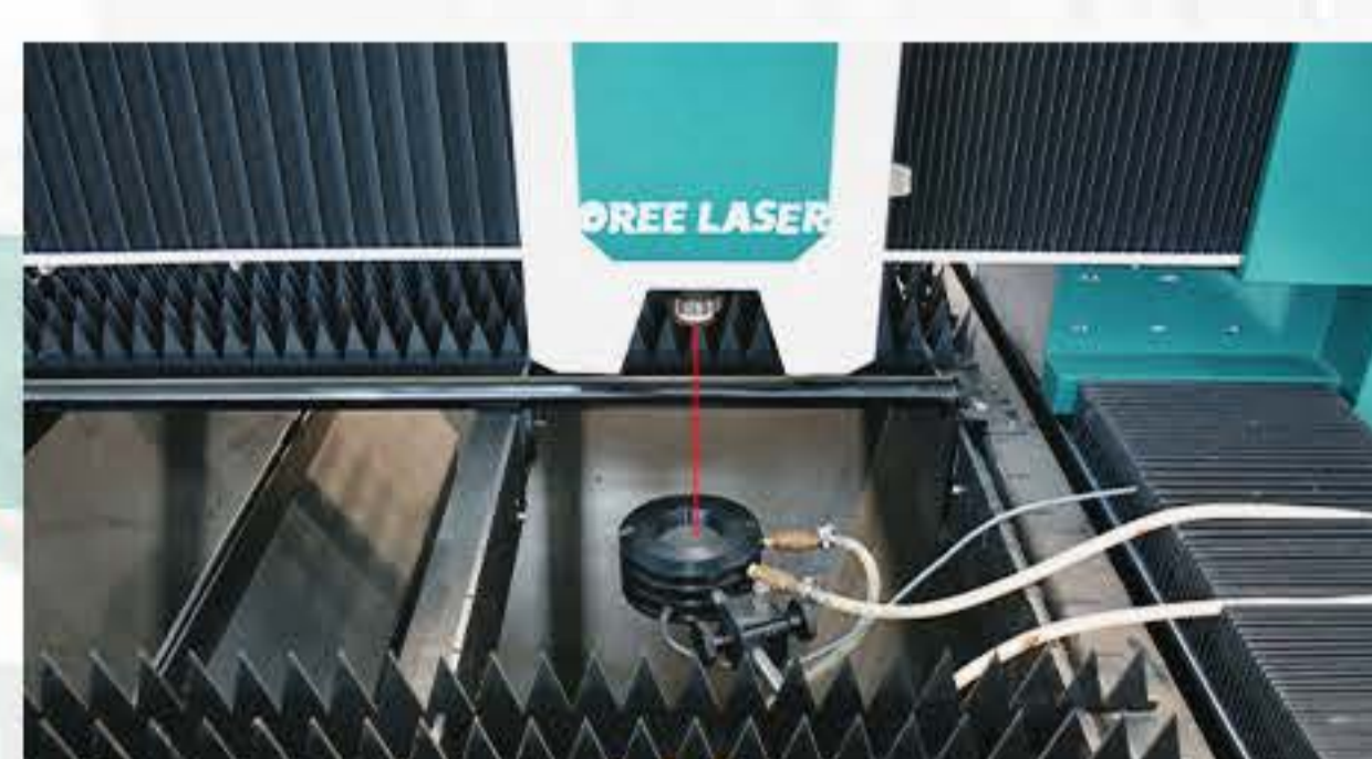
Laser Power Meter Test
