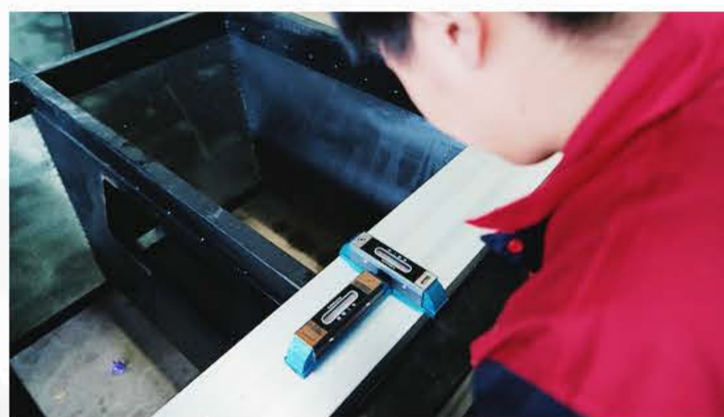
Bed Foot Installation
