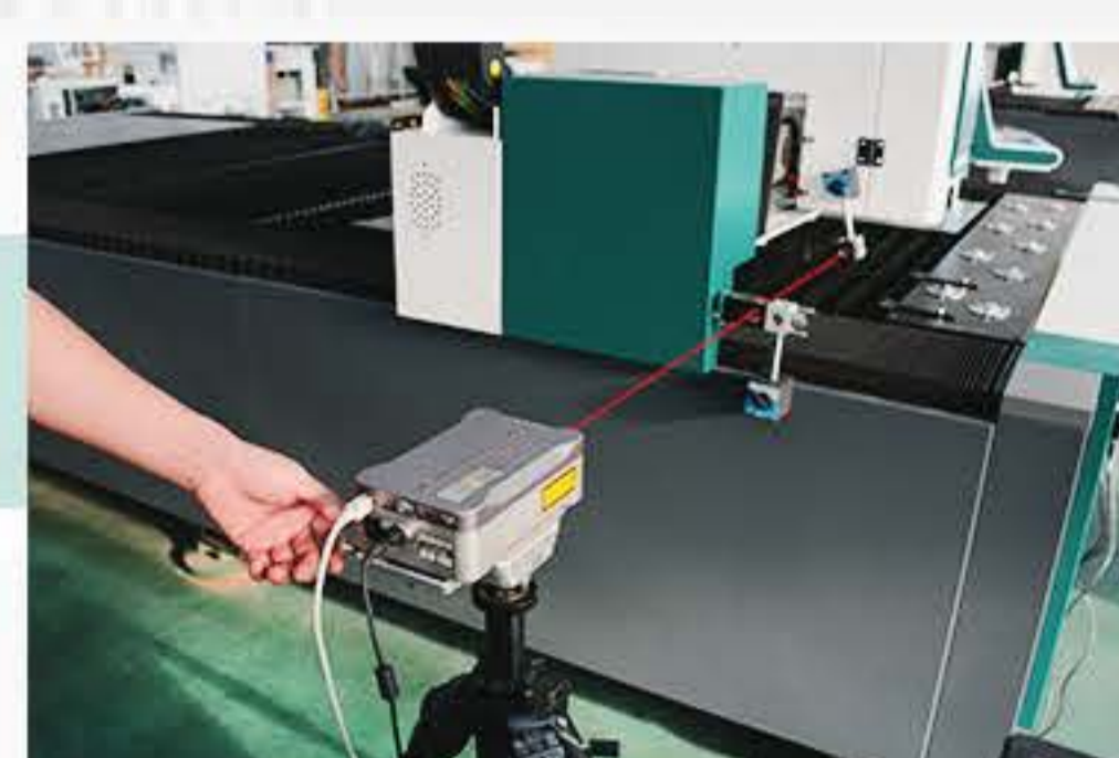
Positioning Accuracy Inspection
