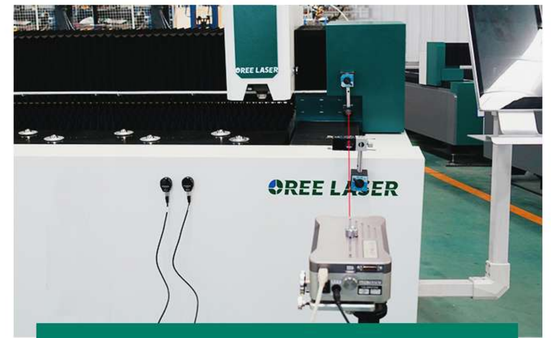
Positioning Accuracy Inspection
