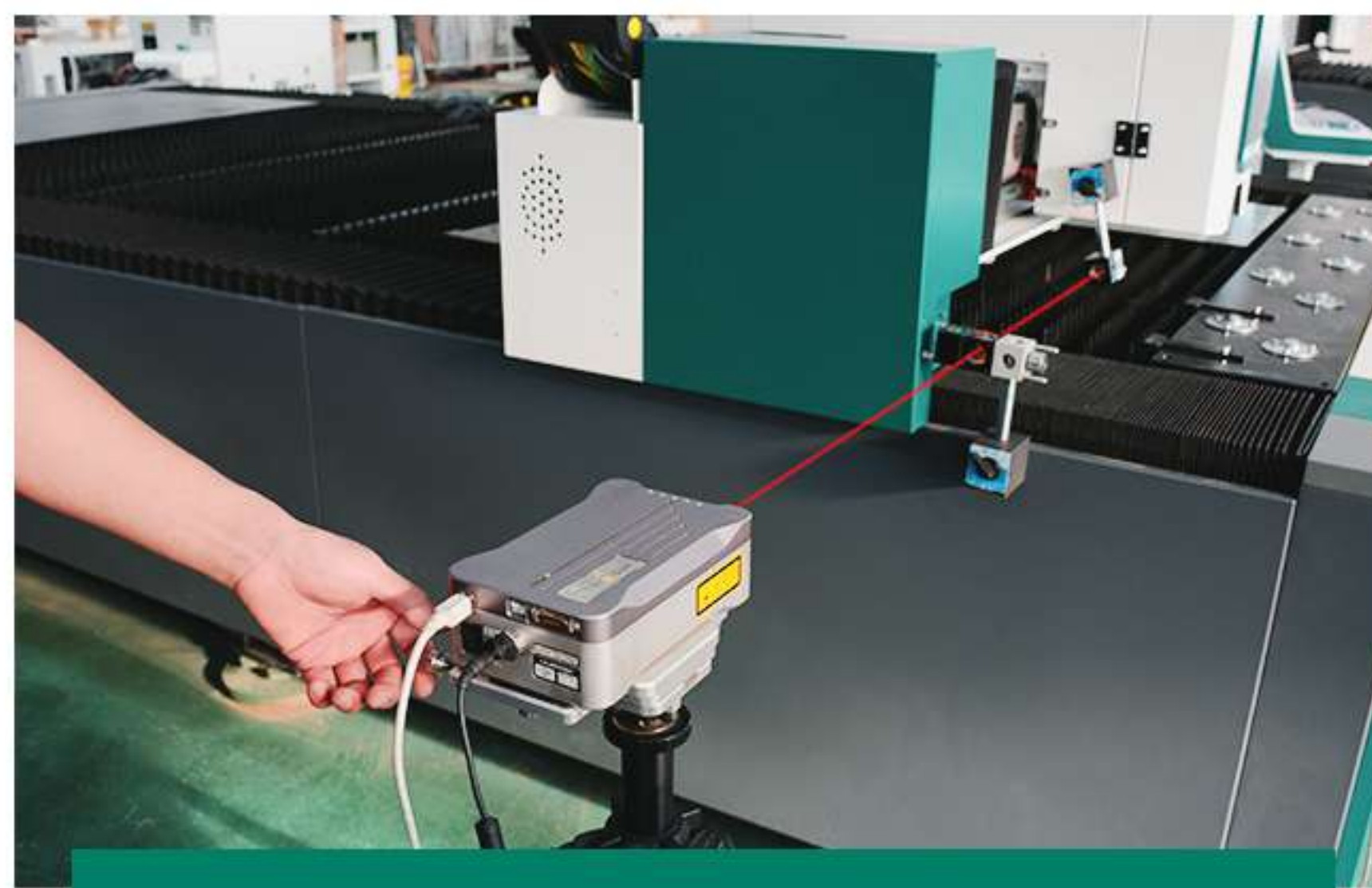
Positioning Accuracy Inspection
