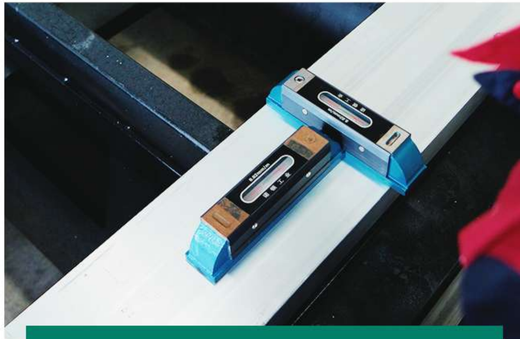
Bed Foot Installation
