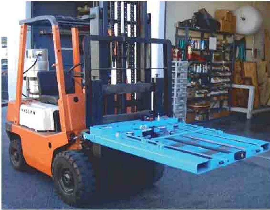
Power Pallet push/pull die loading system, for up to 6,000 lbs
