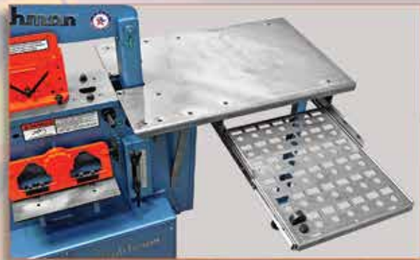
Tool table extension with punch & die drawer
