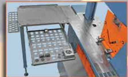
Tool table extension with punch & die drawer
