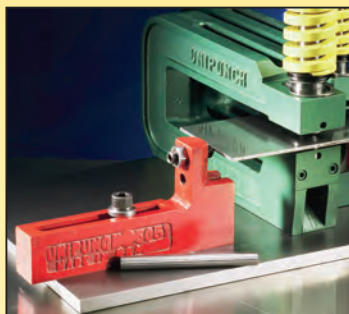
Typical 3-pin gauging Template Mounting
